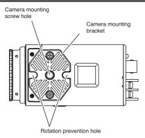
When mounting the camera on a fixer, pan/tilt, etc., use the camera mounting screw hole located on the camera-mounting bracket.
